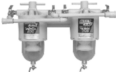
MODEL 200-MFV Double Manifold Diesel Fuel Filter/Water Separator with Shut-Off Valves for Continuous Operation
