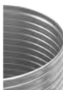
Close-up of deburred edge
