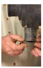
If your air cleaner is equipped with a Donaldson Vacuator™ Valve, make sure your routine filter service includes checking it to make sure it's in good condition and not plugged. If the Vacuator Valve is plugged, clean it.
