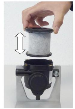
Fig. 11 Changing oil separator of ProVent 100
