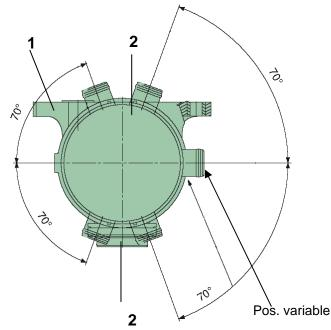
Fig. 4 Positions of outlet for ProVent 150
