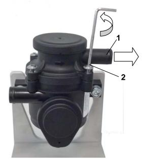
Fig. 10 Detaching lid of ProVent 100
