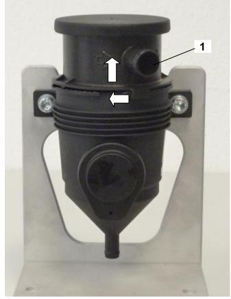
Fig. 12 Detaching lid of ProVent 150
