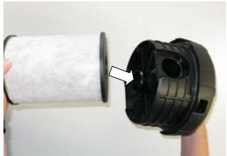
Fig. 24 Fitting oil separator of ProVent 800
