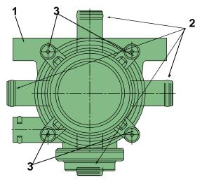
Fig. 3 Positions of outlet for ProVent 100
