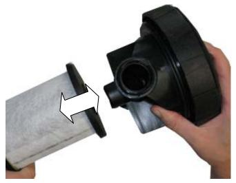
Fig. 19 Changing oil separator of ProVent 400
