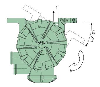
Fig. 5 Positions of outlet for ProVent 200
