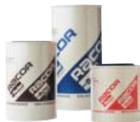
Racor Aquabloc elements are available in 2-, 10- and 30-micron ratings. Red = 30-micron, primary, good. Blue = 10-micron, primary, better. Brown = 2-micron, primary or secondary, best.
