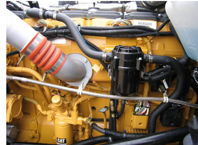
CCV4500 installed on a CAT engine.
