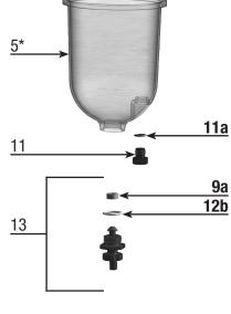
RK 15104 Heat Deflector/Drain Fitting Kit Fits All 900/1000MA Assemblies
