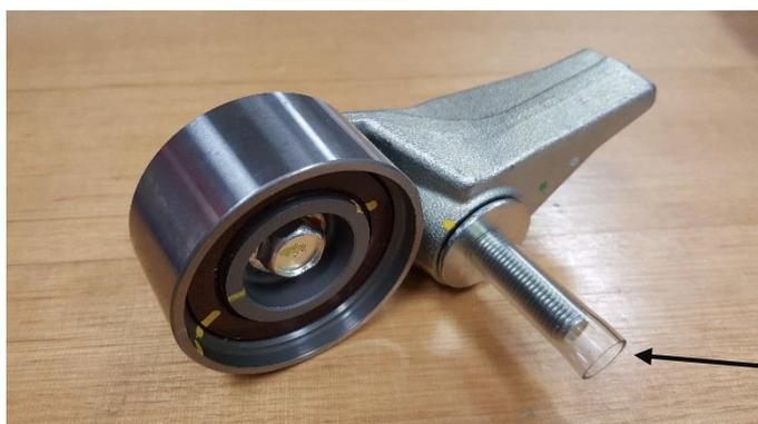
Upon removal of the plastic captive sleeve, it is important that the spacer washer remains in its intended place on the assembly and is included when fitting to the engine. Further, the bolt must be tightened down to a torque of **48Nm +/- 6Nm**. Once fitted, check that the tensioner assembly pivots freely about its mounting point.
