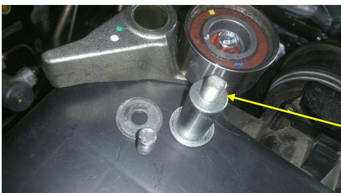
If these additional procedures and checks are not carried out there is a potential for the mounting bolt to fail through fatigue, resulting in engine damage (an example of such a failure shown in photo left). Any claims with evidence of this type of failure will not be covered under warranty.
